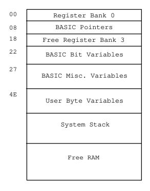
The System Stack is located immediately after the BASIC byte variables. If no byte variables are used, the System Stack begins at 4EH. Free RAM is all the memory above the System Stack. In general, the System Stack should have at least 28H bytes of RAM to use.
